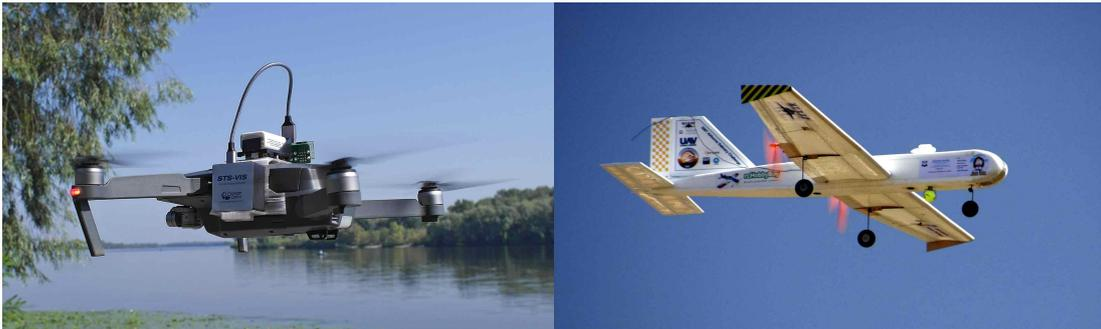
**Figure 2.1:** Two UAV types: rotary (quadcopter, left) and fixed-wing (plane, right)
